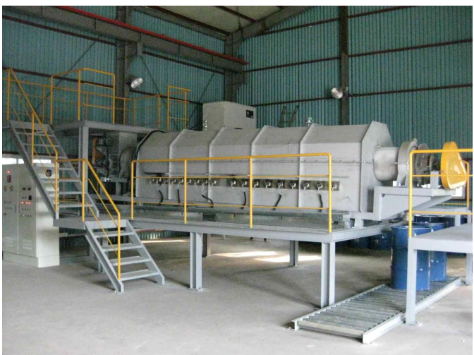
2-15. TMS-Rotary kiln \Phi 560 \times 6,000L 1,000°C
