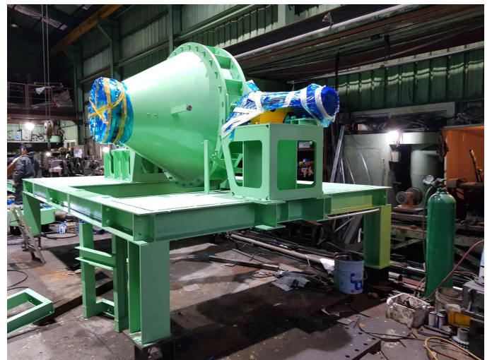
2-22. Rist-Gas burner 80만kcal/hr
