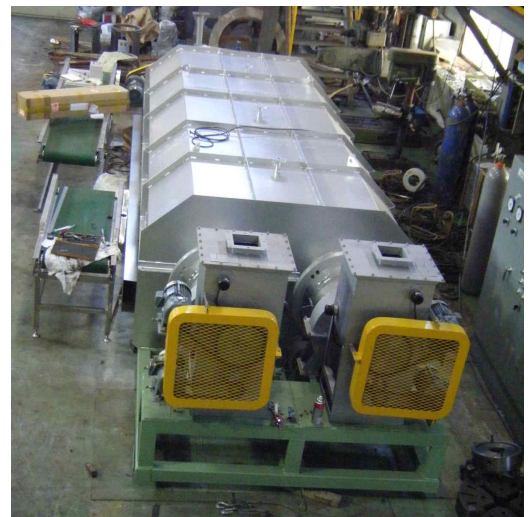
2-7. 삼화화학-Rotary kiln 500 × 2Line
