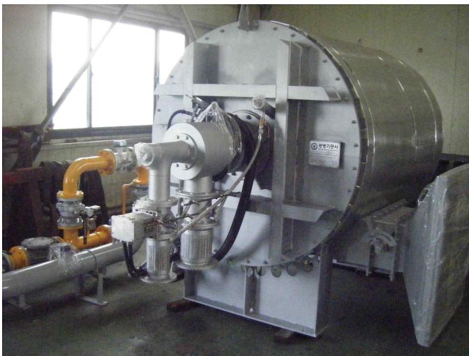
2-15. TMS-Rotary kiln \Phi 560 \times 6,000L 1,000°C
