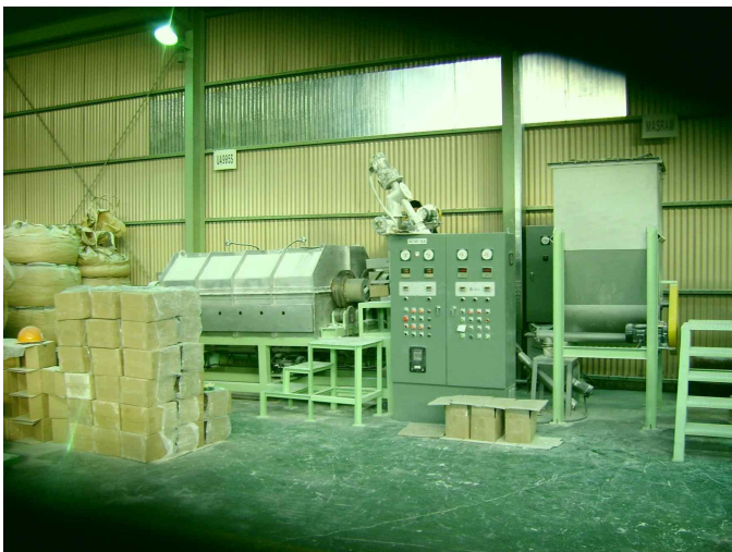
2-7. 삼화화학-Rotary kiln \Phi 250 \times 3,000L \times 2Line 1,000°C
