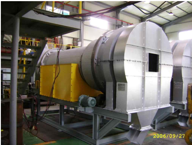
2-7. 삼화화학-Rotary kiln \Phi 250 \times 3,000L \times 2Line 1,000°C
