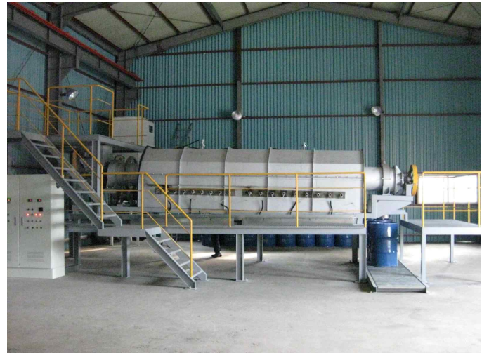
2-15. TMS-Rotary kiln \Phi 560 \times 6,000L 1,000°C
